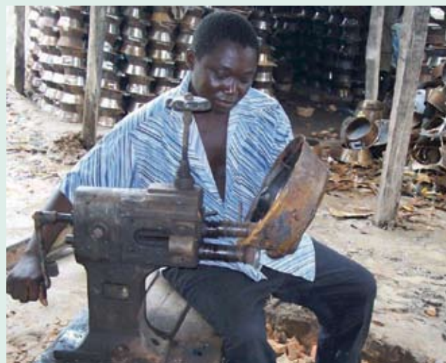
Photo 31: Sahara (A) group chairman Hamisi Nasoro, shaping a metal cladding using pottery heel machine
