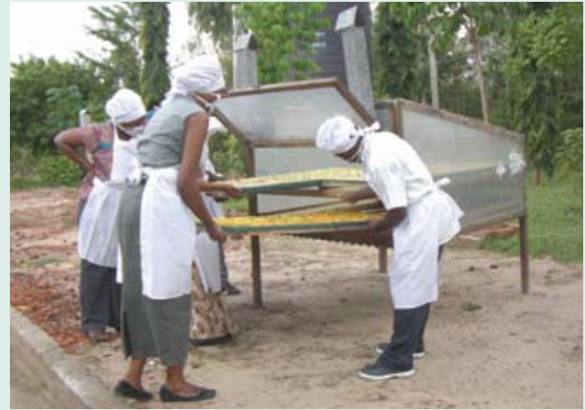
Photo 25: The participants of solar drying training during a practical session put trays of fruits in the solar dryer
