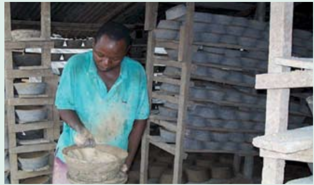
Photo 32: Mr Japo Nasoro making liner at the Sahara (A) workshop
