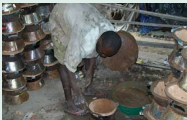
Photo 30: An artisan finalizing an improved charcoal stove at Sahara A. Group Workshop in Vingunguti, Dar es Salaam
