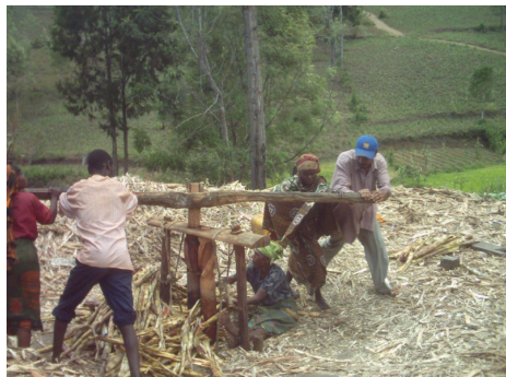
Typical traditional sugarcane juice extractor (mkoroto) for local beer processing can be replaced with sugar cane pressing motor powered by micro electric hydropower.
